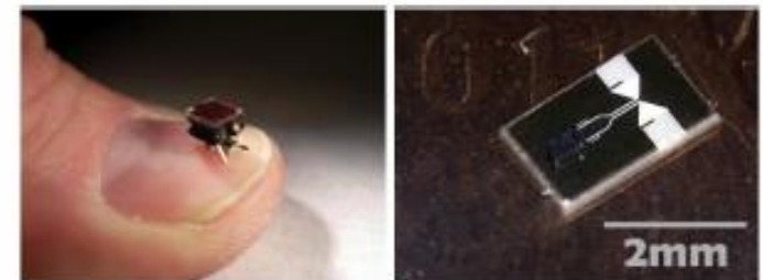
Fig. 1: (a) Photograph of the I-SWARM micro-robot [1], (b) Proposed 94GHz rectenna.
