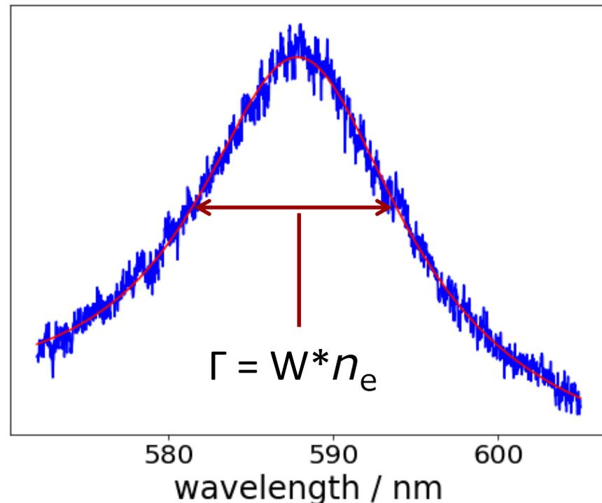
0.2 atm Ar in which ArII spectral lines were visible
