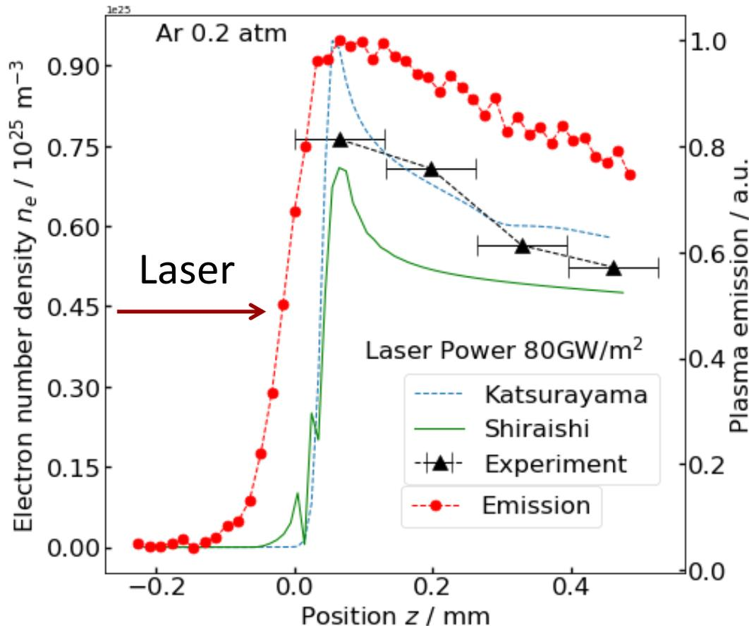
Emission and  $n_e$  distribution from experiment and simulations
