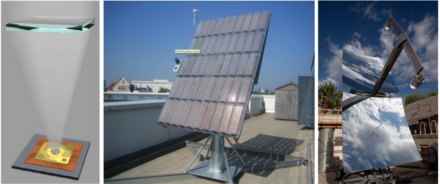
Figure 1: Left and middle: Example of a CPV system using Fresnel lenses to concentrate the sunlight: FLATCON ® concept originally developed at Fraunhofer ISE. Right: Example of a mirror-based system developed by the University of Arizona, USA [7].
