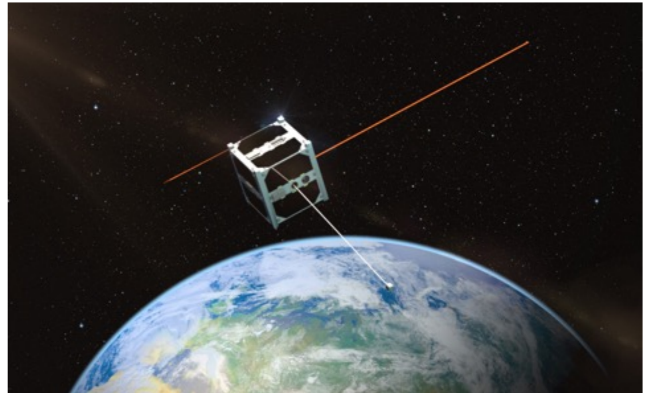
ESTCube-1 (1 kg nano-sat): the first satellite to test electric sail 1
