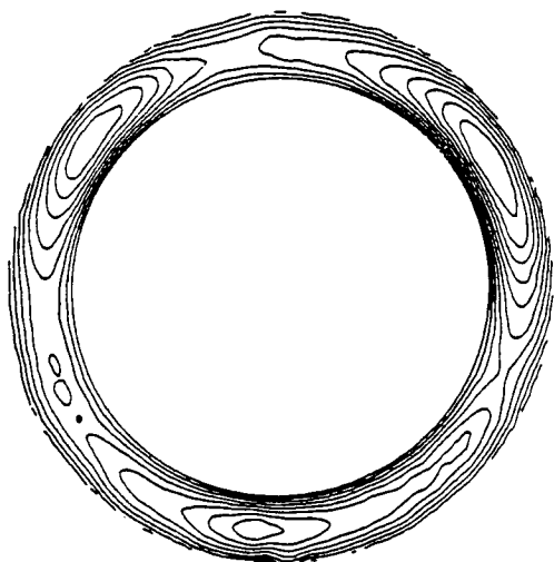
Fig. 24 Contour of the space potential in the acceleration channel.
