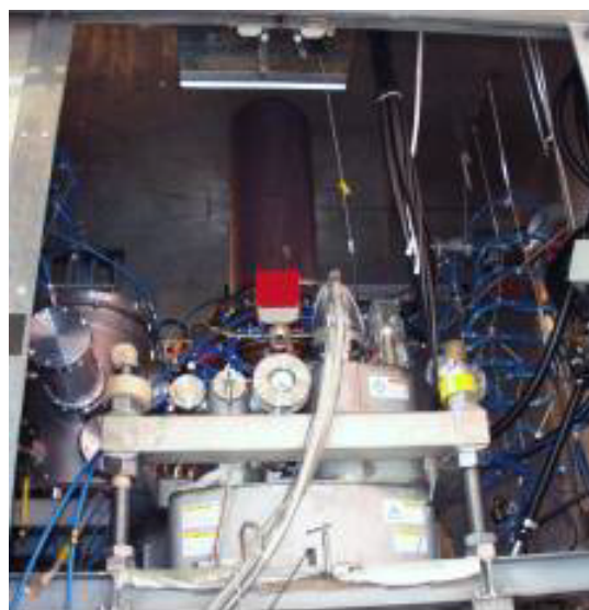
Fig. 1 The gyrotron developed at the Japan Atomic Energy Research Institute.
