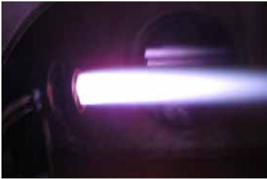
**Figure 12. Photo of zirconia cathode arc-heater plume**
