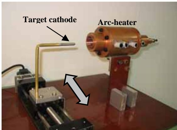
Figure 10. Oxidation system
