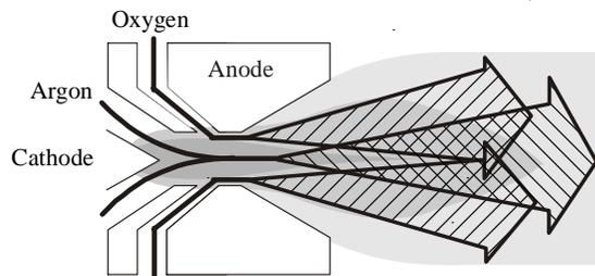
Figure 4. Mixing process.
