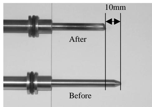
**Figure 9. Cathode erosion (one hour off and on operation).**
