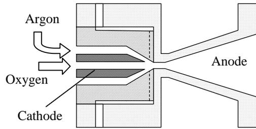
**Figure 5. Hollow cathode arc-heater.**
