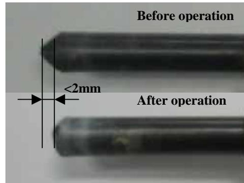
**Figure 13. Zirconia cathode before and after twenty minutes operation**
