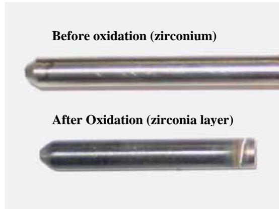
Figure 11. Zirconium cathode before and after oxidation
