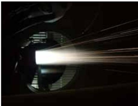
**Figure 8. Photo of unstable hollow cathode arc-heater plume.**
