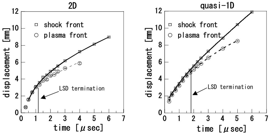
Figure 4: Displacements of the shock wave and plasma front. 2D LSD and quasi-1D LSD.
