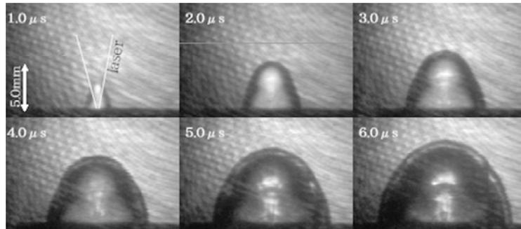
Figure 1: Shadowgraphs of the 2D LSD wave evolution.
