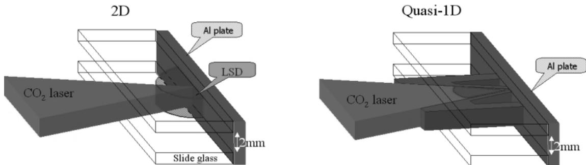
Figure 6: Laser focusing apparatus for LSD wave visualization.
