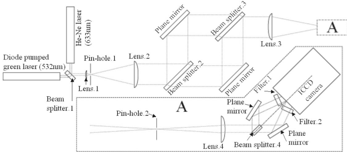
Figure 7: The two-wavelength Mach-Zehnder interferometry system.
