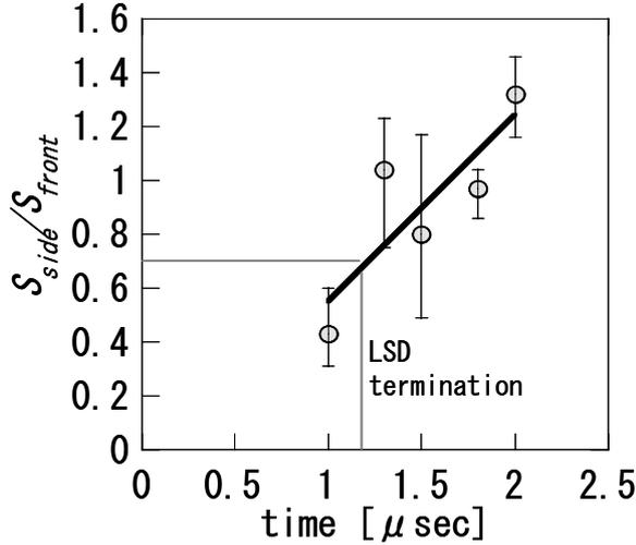
Figure 10: Measured  $S_{\text{side}}/S_{\text{front}}$  in 2D LSD case.
