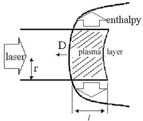
Figure 5: The conceptual rendering of Raizer's LSD termination theory.
