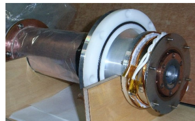
Fig.32 An MPDT with an extended support. This structure is for the optical measurement at the MPD muzzle.
