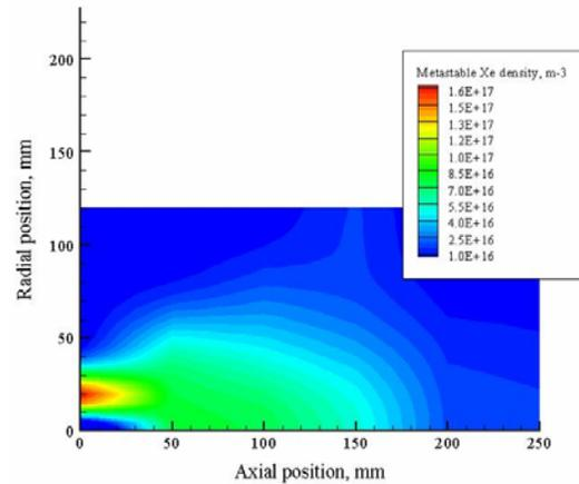
**Fig. 6** Number density distribution of meta-stable xenon atom in the normal pressure condition.
