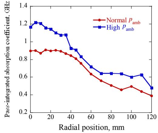
**Fig. 5** Distributions of pass-integrated absorption coefficients at different ambient pressure,  $z=20$ mm.
