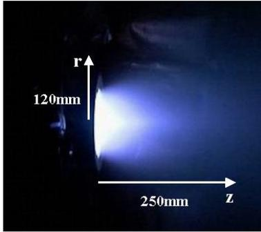
**Fig. 2 A photo of a Hall thruster plume.**
