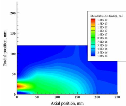
**Fig. 6** Number density distribution of meta-stable xenon atom in the normal pressure condition.
