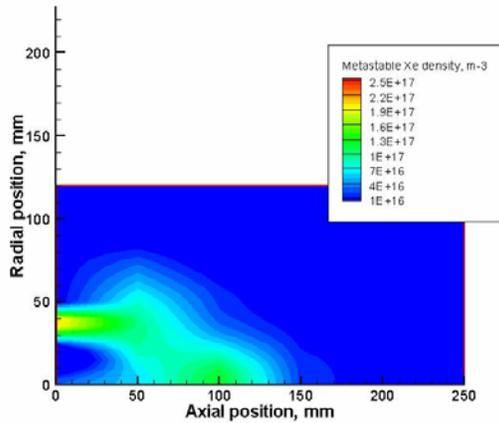
**Fig. 7** Number density distribution of ambient xenon.
