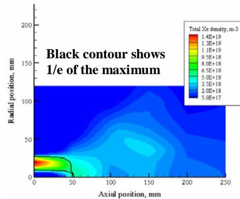
**Fig. 8** Number density distribution of total propellant xenon atom.
