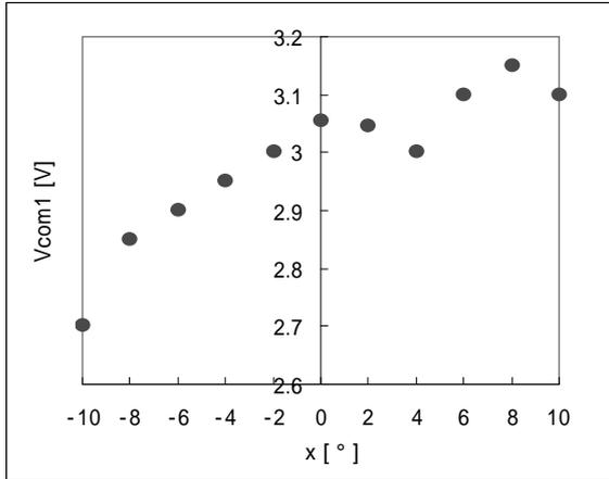
**Fig.12. The output voltage while the transmitter antenna was shifted in x axis. (y=0)**
