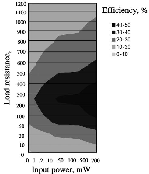
**Fig. 5 Rectification efficiency.**
