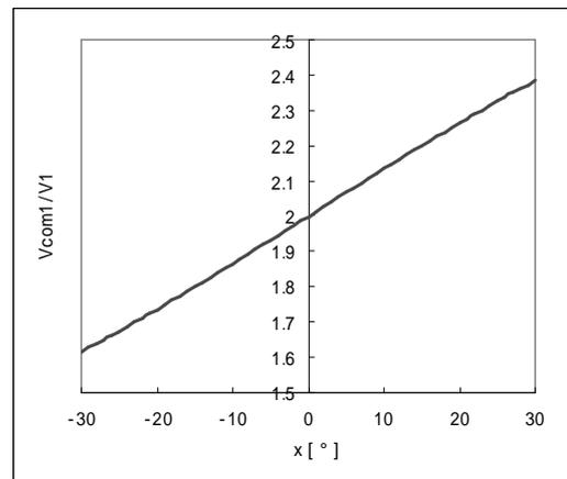
Fig. 9. Expected relationship between incident angle  $\alpha$  and output signal  $V_{com1} / V_1$ .
