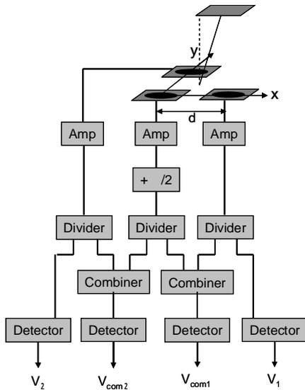
Fig. 8. The block diagram of tracking system.
