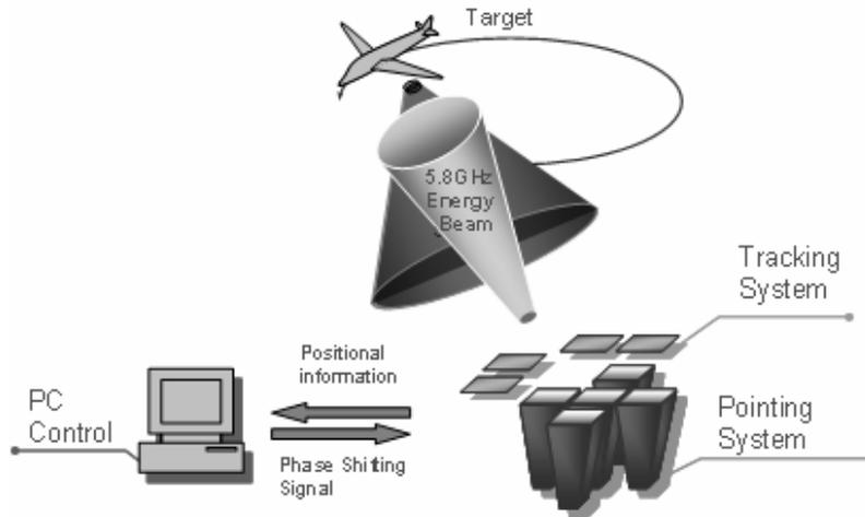
**Figure 1. Schematic of the microwave power supply system to MAV.**
