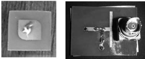
**Fig. 4 A patch antennas for circular polarization (left) and rectifier circuit (right).**
