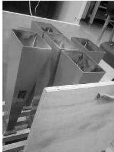
**Fig. 3. The picture of the five arrayed antenna elements.**
