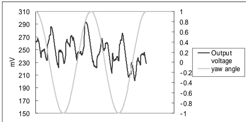
**Fig.11. Rectenna output voltage and difference between yaw angle and direction of linearly-polarized wave while the microwave beam synchronized the MAV**
