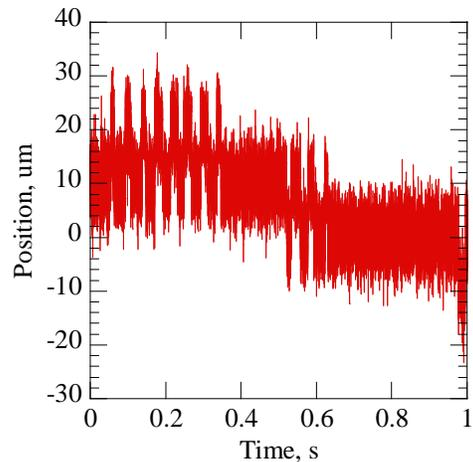
Fig.6 The mechanical vibration of the vacuum chamber for Arc heated wind tunnel
