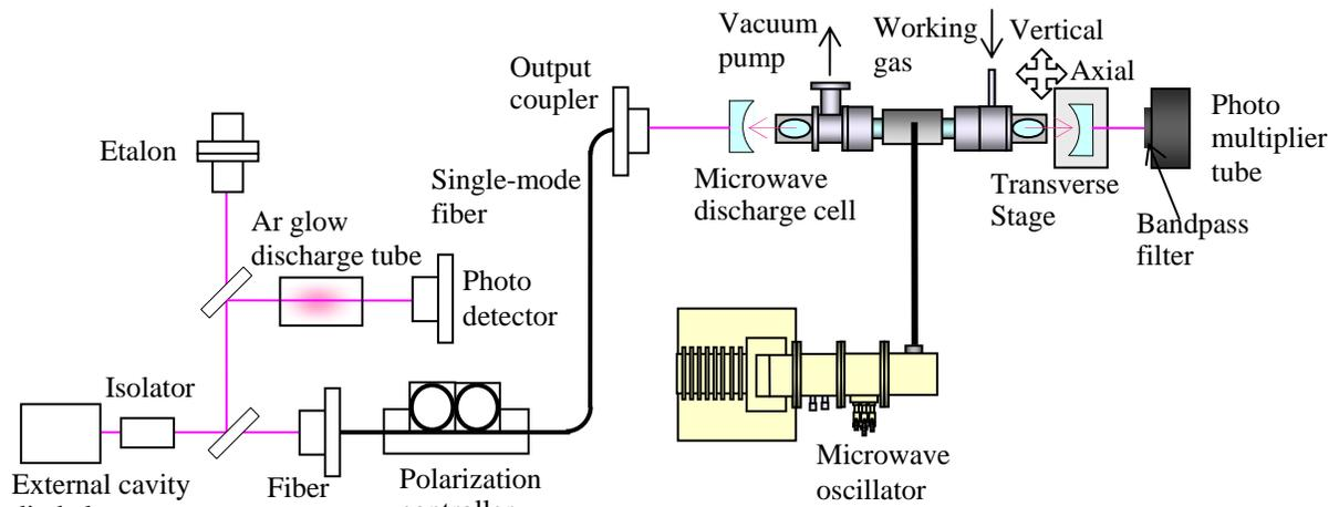
Fig.4 The schematic of measurement system for cavity enhanced absorption spectroscopy
