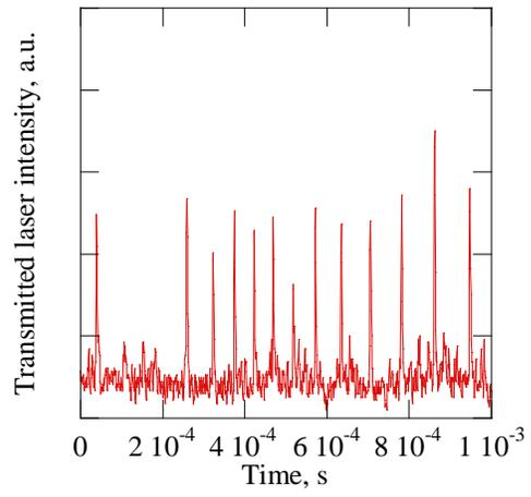
(b) Axial vibration with 5,000GHz/s sweep
