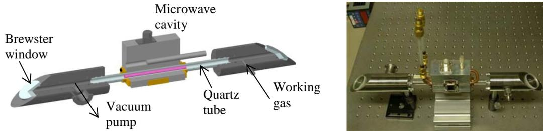
Fig.3 The schematic of the microwave discharge cell (left) and its photograph (right)
