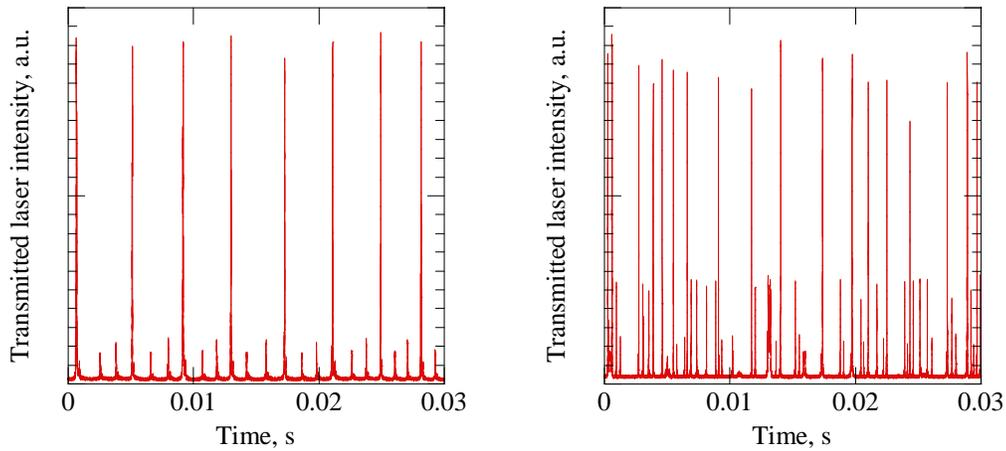
Fig.1 Transmitted laser intensity through the cavity without (left) and with (right) the working of the vacuum pump and cooling water
