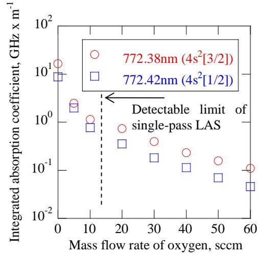
Fig. 6 Integrated absorption coefficient of the microwave discharge cell
