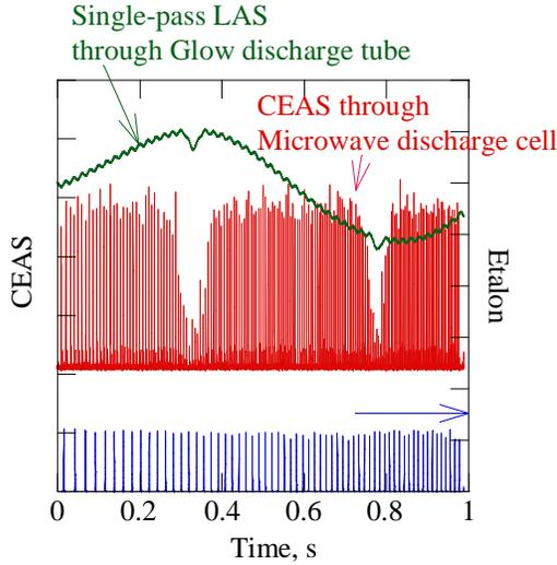
Fig.5 CEAS signal of atomic argon generated by microwave discharge tube, single-pass LAS signal in the glow discharge tube and etalon signal
