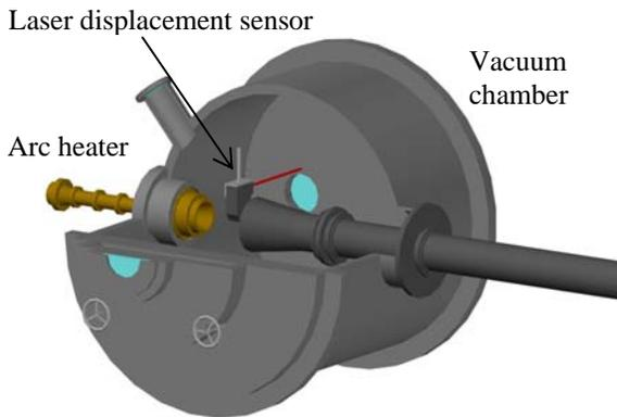
Fig.5 Experimental setup for the measurement of the mechanical vibration of the vacuum chamber for Arc heated wind tunnel
