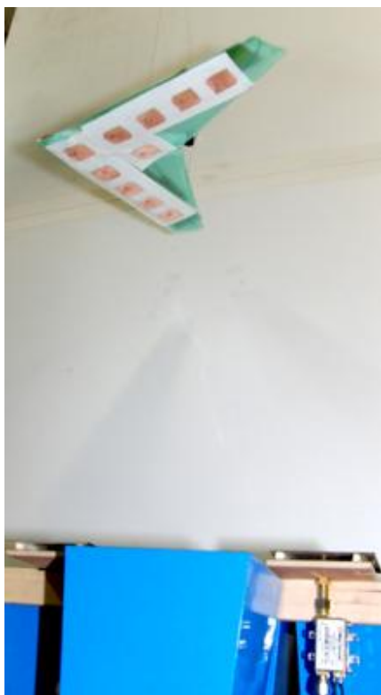
Figure 1 Micro Aerial vehicle model above a microwave power transmitter. Patch rectenna array is mounted.
