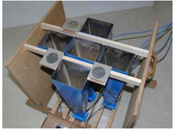
Figure 6 Integration of the transmitter antennas and tracking antennas.
